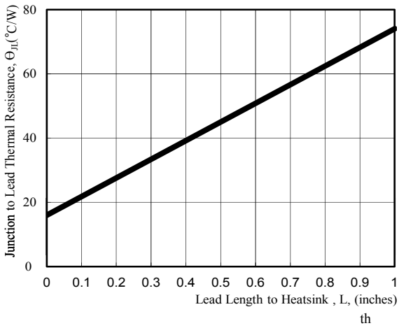
Fig. 5 - Typical Thermal Response L, Lead Length=3/8inch
